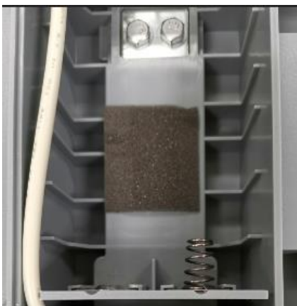
Figure 3-7. Removing bolts holding Frame to the bottom housing
