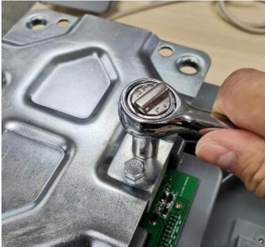
Figure 3-6. Removing bolts holding Frame to the Load Cell.
