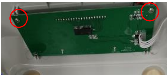
Figure 3-5 Rear Display PCB.
